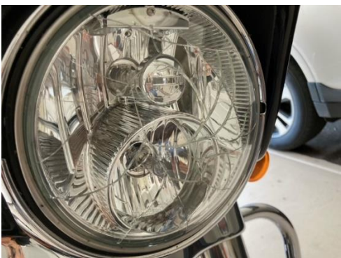
Cracked Headlamp-Look Closely. See Cracks all Over!
